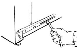
Pull firmly to remove the other end of shipping strap from the back of the washer. The shipping strap plug must be completely removed from the washer for the self-leveling legs to be released.
